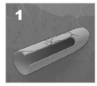
After cleaning and evaluating the existing pipe for damage, the sewer pipe is ready for its new lining.
